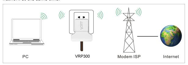
3. Intelligent wifi bridge mode(VRP300): WiFi intelligent bridge function, wireless to wired, wired to wireless intelligent switching
